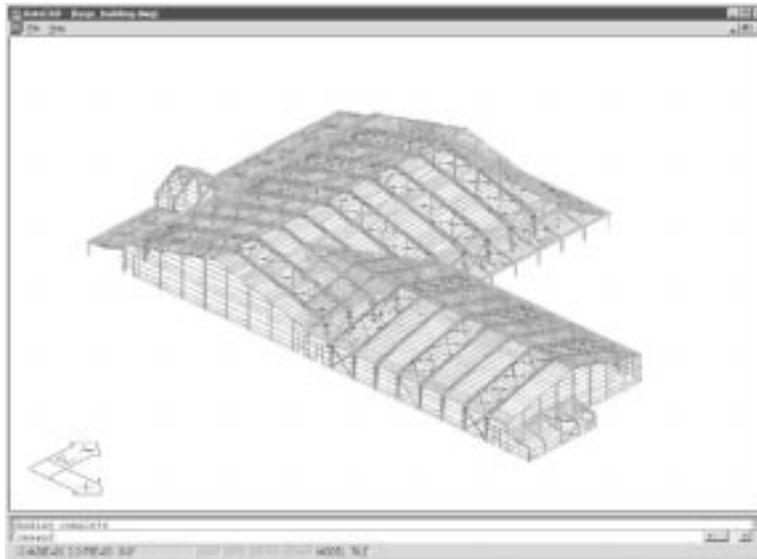
Figure 3. Robertson Ceco Corp. uses a knowledge-based ETO configuration system to create custom building designs.
